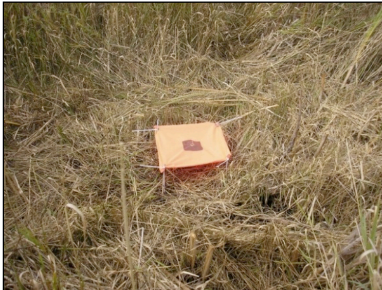
Figure 13 A deployed ground control point (GCP). Photograph by T. Bowron, September 2010.
