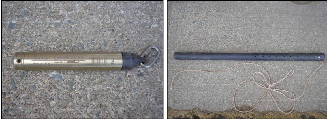
Figure 14 Solinst Levelogger (model 3001) on the left and still well on the right. Photographs by N. Neatt, 2007.
