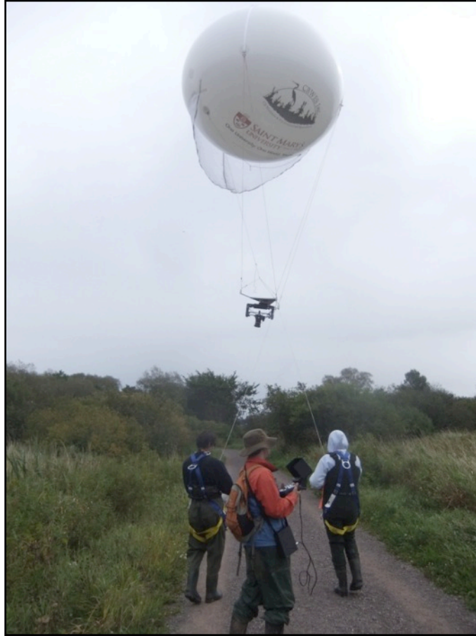
Figure 12 The CBWES-SMU helium blimp and remote operated suspended camera system used to capture low-altitude geo-referenced air photographs. Photograph by T. Bowron, September 2010.
